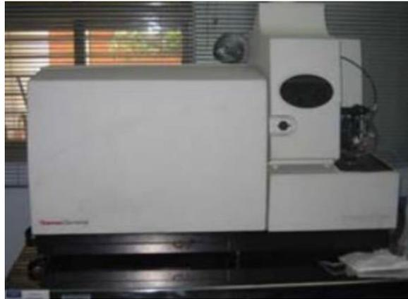
**Gambar 2.1 Instrument ICP-MS (Septiani, 2021)**
